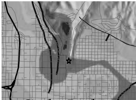
Figure 2 – Excerpt - Ground Shaking Map from Wong 2002. Notes: The proposed DPU facility is marked with a star in an MMI IX predicted shaking region. The faults to the immediate west are extensions of the Warm Springs Fault and have been active in the last 15, 000 years.
